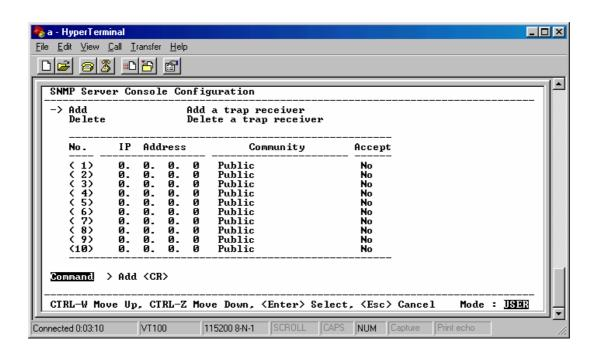
18. Arrow down to Trap and hit enter. This screen allows the user to send Traps about the UPS to ten IP Addresses (not required). Also, you may determine the severity levels and what type of access, read only or read and write, to assign to a particular IP manager. Hit the "Escape" key to return to the main menu.
